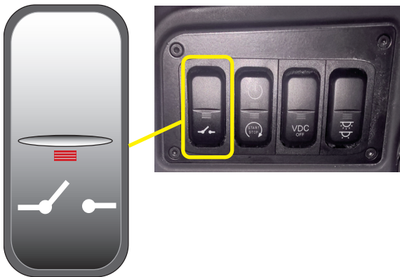
Master Switch on Drivers Dashboard
