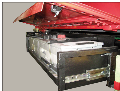
Vehicle 24V DC Battery tray extended
