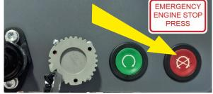
An engine emergency STOP is fitted inside a flap at the rear right hand side of the vehicle.
