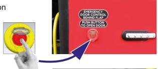
To open the door from inside, push the emergency button located near the top edge of the doors.
